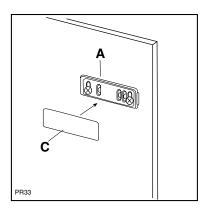
Open the appliance door and the furniture door at 90°. Insert the small square (B) into guide (A). Put together the appliance door and the furniture door and mark the holes as indicated in the figure. Remove the squares and drill holes with  $\emptyset$  2 mm at 8 mm from the outer edge of the door. Place the small square on the guide again and fix it with the screws supplied.
